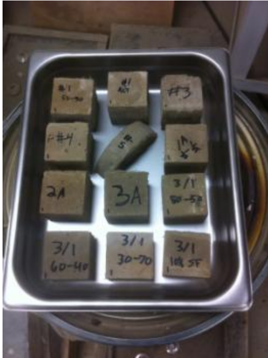
Figure 6.4: Specimens before heating to 585°C
