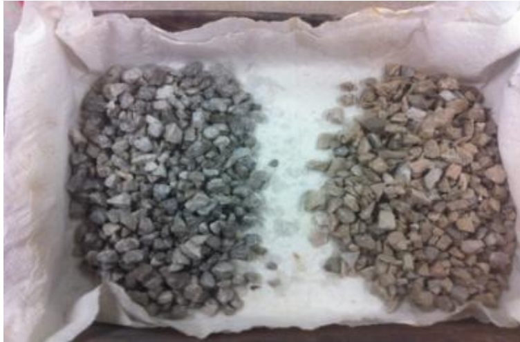
Figure 6.2: Limestone before (left) and after (right) 500 hours at 550°C
