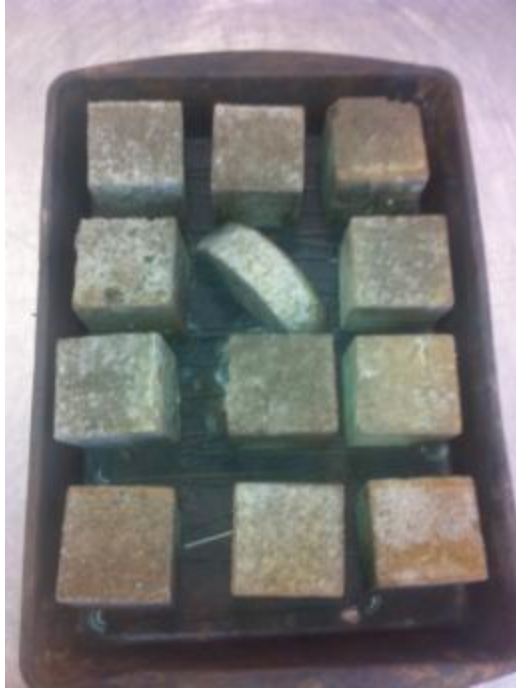
Figure 6.5: Specimens after heating to 585°C for 500 hours
