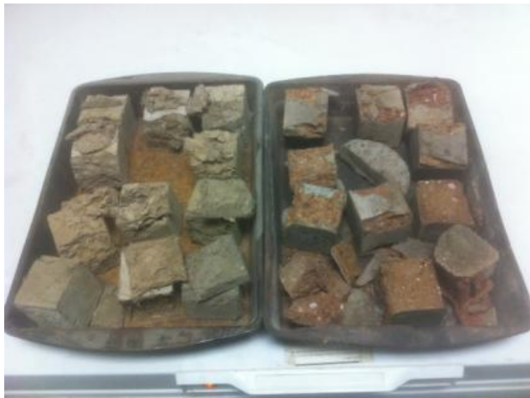
Figure 6.7: Concrete cubes before (left) and after (right) 500 hours at 585°C
